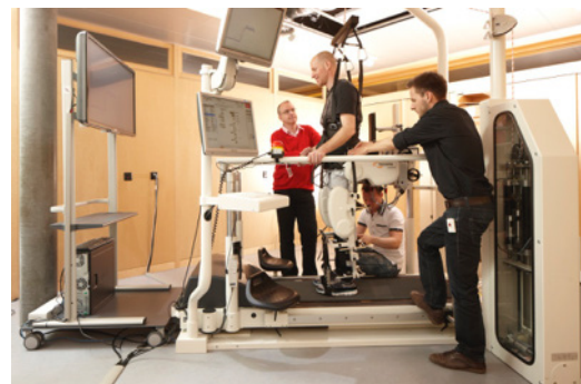
Fig. 2: Lokomat exoskeleton rehabilitation robot.
