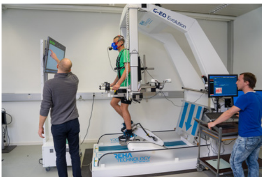
Fig. 1: G-EO System end-effector rehabilitation robot
